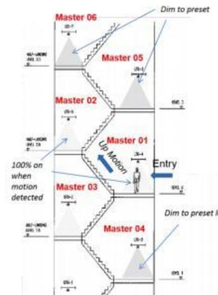
**Dual Technology ( BT + Microwave) in Dimming Control**
